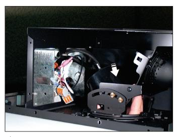
Pull the transformer out of the housing. Do not disconnect any wires at this time. The wires have enough slack to pull the transformer completely out without disconnecting.
