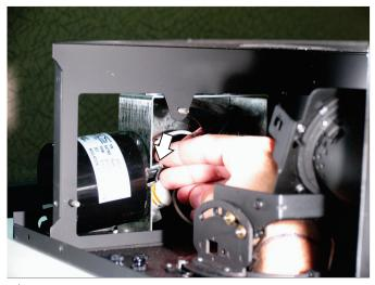
Remove the large wing nut inside the electrical box. This wing nut holds the transformer in place.
